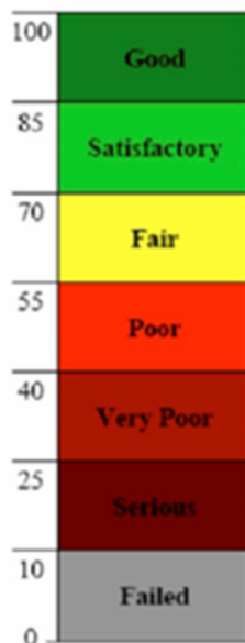
Figure 1: ASTM Pavement Condition
